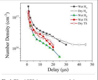
**Fig. 1**. TS and OES time measurement of plasma kinetics with and without water vapor electron number density.
